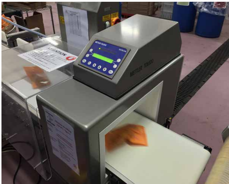
At the lines the installed critical controlpoints (CCP's) check all packages against metal contamination to ensure their product safety according to IFS guidelines.
