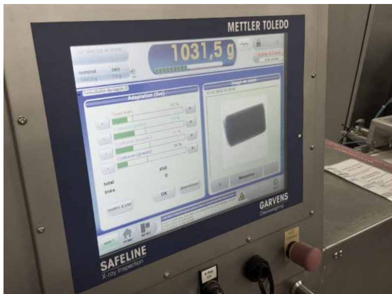
The software user interface of the combination system shows both, the result of the weighing and x-ray inspection.
